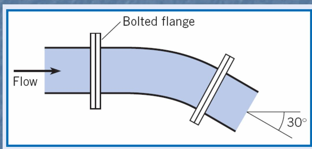
Find the force required to hold the bend in place?
